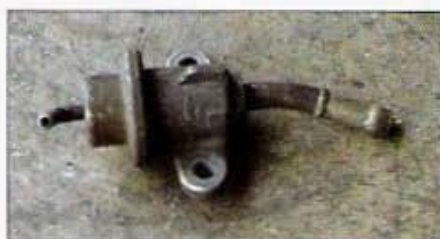
The fuel regulator outlet in this case is slightly larger than the return line found on the Civic. A reducer will need to be used in between the two hoses in order to make the connection.
