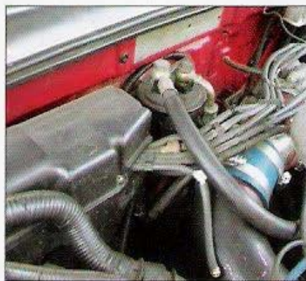
In this case, the original Prelude fuel injection feed hose simply reattaches to the new Prelude fuel rail. Be sure to replace the crush washers for the ultimate seal.
