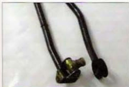
This custom-fabricated shift linkage from HCP Engineering will provide you with the simplest install. Notice the Integra-style ends in the lower portion of the photo.
