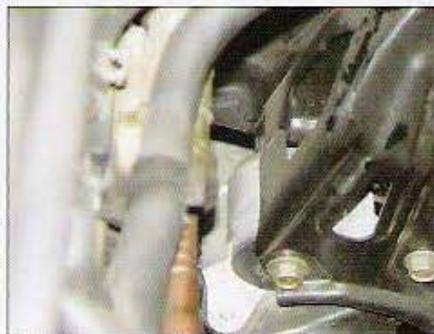
Once the subframe is raised into position, the rear bracket of the K-series can be attached to the mount and bolted down. (Photo Courtesy of Hasport Performance)
