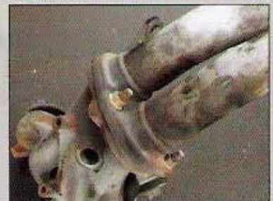
Notice where the downpipe connects to the upper portion of the exhaust manifold. Often times the bolt pattern differs between manifolds that you would assume would be similar.
