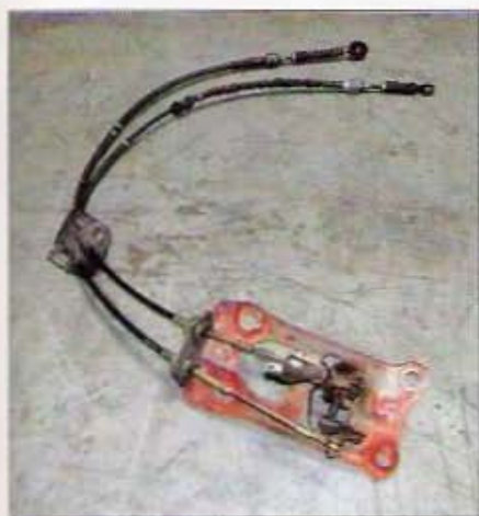
Many shifter cables look alike. These were purchased as a unit from a local wrecking yard. They came from a '92-'96 Prelude with the manual transmission.
