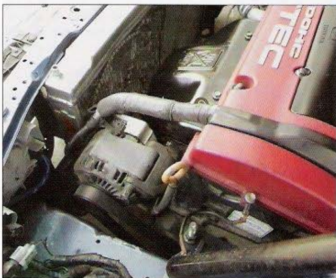
An uncommon sight to say the least, you won't find many H22A swaps into the '88-'91 Prelude chassis.
