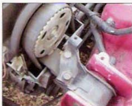
A combination of the '92-'95 Civic engine bracket and '88-'91 Civic engine mount will adapt this late-model D series into the older chassis.
