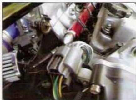
All SOHC VTEC engines are OBD I or II. That means you'll need to modify the late-model distributor for use with the old engine harness. Simply swap the plugs from the donor engine onto the Civic harness.
