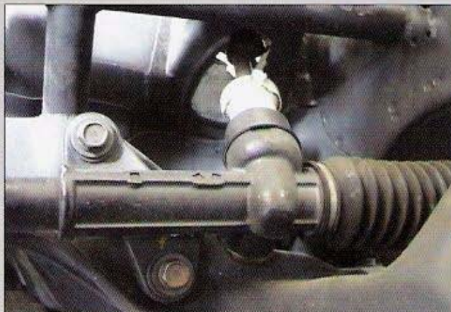
Ideally, the right way to get rid of your power steering is just to swap in a manual steering rack, like this one.
