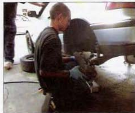
Eric Cardines of Honda Fiend is seen here installing a set of Integra rear brakes and trailing arms. Although it isn't necessary on the D-series swap, a brake upgrade is never a bad idea.
