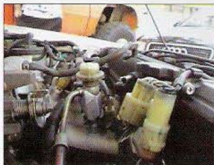
Often, distributor connectors need to be swapped out for those of the donor engine. Attach the plugs to the old harness by removing the pins or cutting and soldering the wires.
