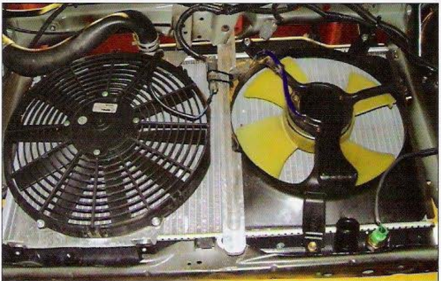
Here's a look at the '02-'03 Civic Si radiator installed into this Civic. If you look toward the top, you can see where it had interfered with the hood latch. (Photo Courtesy of Hasport Performance)
