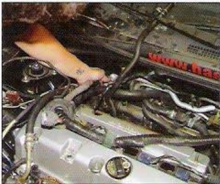
The wiring is being positioned onto the engine and fished into the vehicle in this photo. A custom harness from Hasport Performance was used because the electrical system is fairly complex on this swap. (Photo Courtesy of Hasport Performance)
