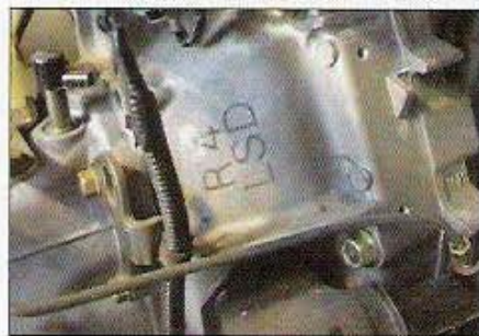
Generally, limited-slip-differential (LSD) transmissions are labeled as such. If you want to know for sure, simply look inside the axle orifice on either side of the unit. On LSD-equipped transmissions, you can see straight through, while the standard units will have a shaft in the middle.
