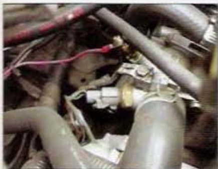
Since the fan switch is in a different location on the donor engine, you'll need to lengthen the wires from their original position, which was on the back of the engine block.
