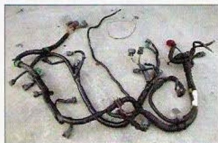
The wires for VTEC were just added. They exit the center of this harness and make their way upward. Running them as part of the original harness makes for a factory look.
