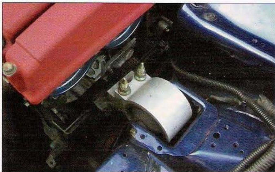
Once the correct post mount is installed, in certain cases you can reuse the original Civic or Integra engine mount on the driver side of the vehicle.
