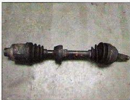
Custom-length axles will be mandatory for this swap, and the joint that attaches to the intermediate shaft may differ. Since this setup uses a late-model half shaft, it requires the corresponding late-model axle with the female end.
