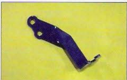
This special throttle-cable bracket from Place Racing will allow you to reuse the original Prelude throttle cable. It simply bolts onto the intake manifold.
