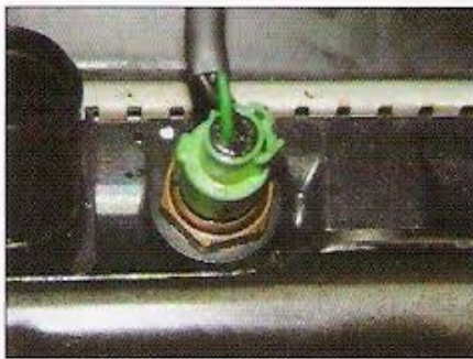
The ECT (engine coolant temperature) switch wiring must be lengthened on the Civic harness if you're installing the Civic Si radiator. This is the new location of the plug on the new radiator. (Photo Courtesy of Hasport Performance)
