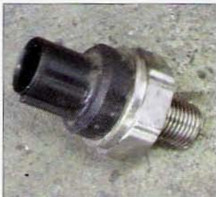
Almost all VTEC engines require a knock sensor. If you don't wire it up properly, you'll get a check-engine light and VTEC won't work correctly.
