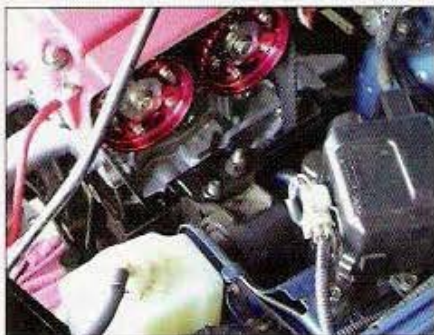
This late-model B16A will fit perfectly reusing both the post mount and the engine mount of the B18A engine.
