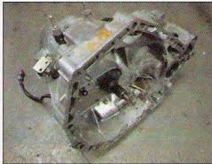
This late-model Integra hydraulic transmission can be identified by the style of its input shaft. These hydro units also feature studs on the top to which the top mount is attached.
