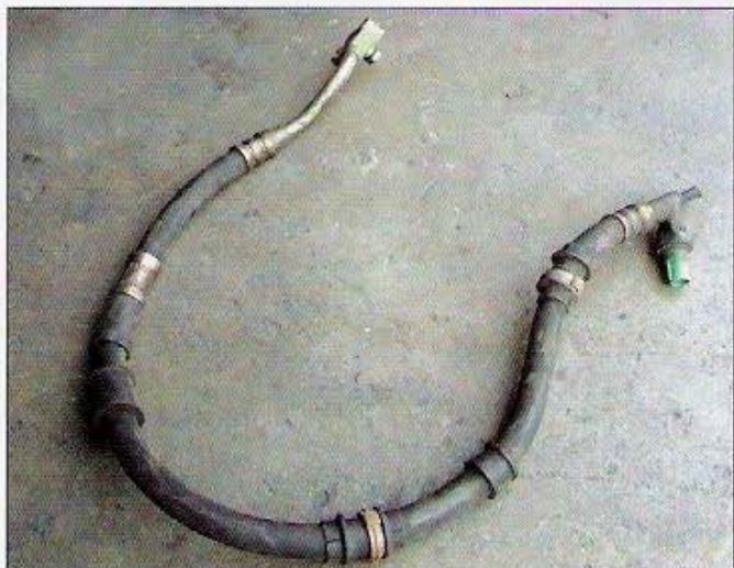
Often, power-steering hoses such as these may be acquired from a junkyard engine.
