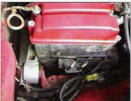
This Hasport Performance left-side engine mount bolts perfectly into place. This is one of the only B-series engine transplants where the OEM bracket in the middle of the picture will not be used.
