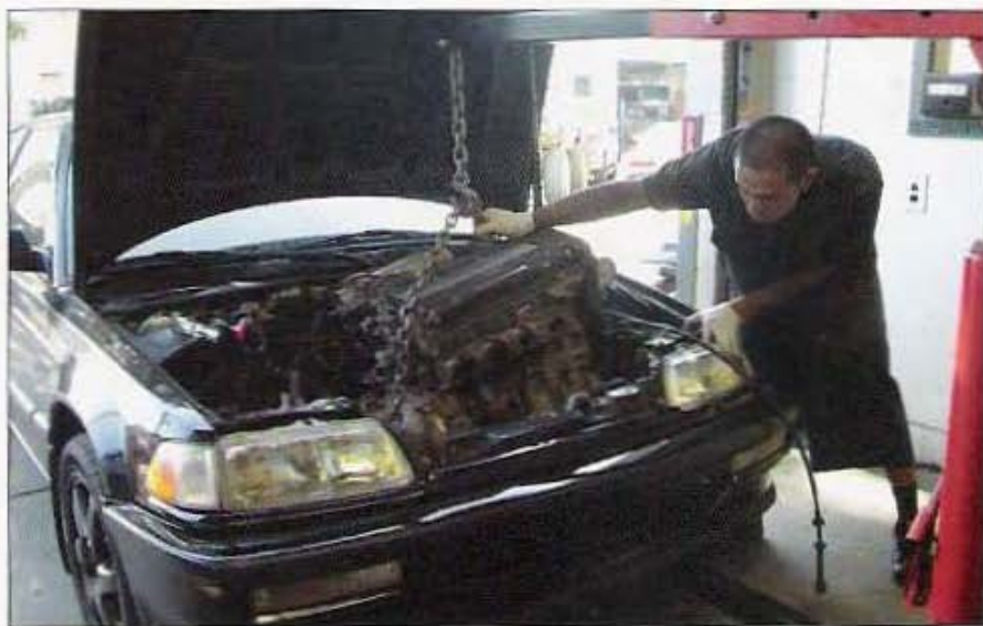
Lowering the engine down at an angle, Cardines of Honda Fiend Racing gives it one final look to make sure the new engine isn't going to hit anything on its way down.
