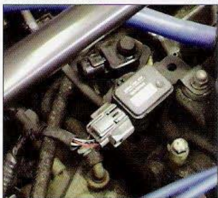
Rather than mounting it on the firewall, the owner chose to mount this MAP sensor to the valve cover for a tidy look.
