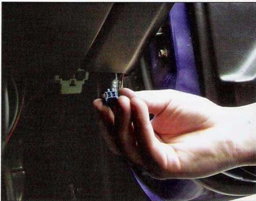
The connector is located just behind the glove box on the '94-'01 Integra. Use a paper clip or piece of wire to jump the two terminals in this connector if you want to read the trouble codes on the dash.
