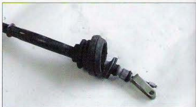
Install the new Integra clutch cable underneath the dashboard of the Civic with this special clip. There's no way around this one; it must be swapped out.
