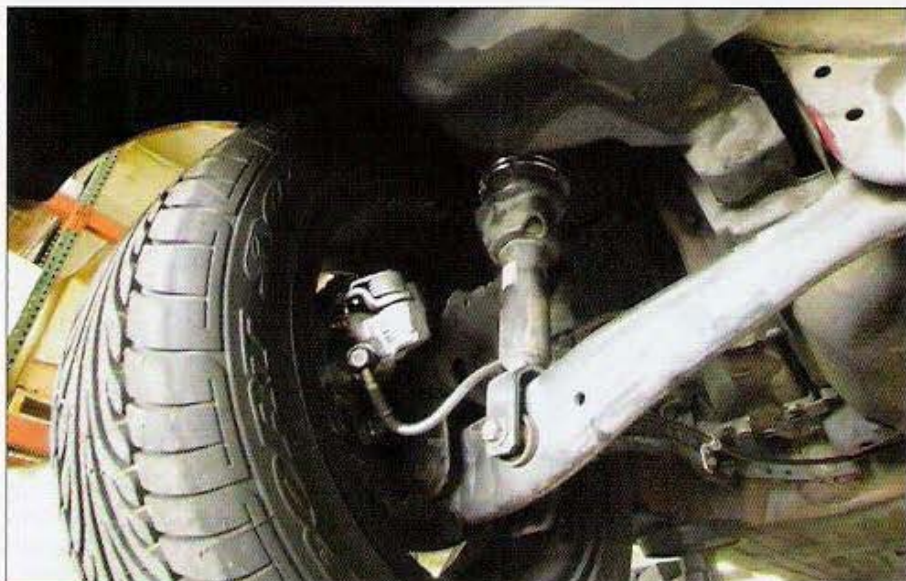
Notice how the rear brakes were converted with components from a late-model Integra. You can see the larger calipers on the back portion of the rotor.
