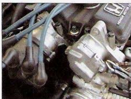
Since the cylinder position sensor is driven off of the exhaust camshaft on the B20A5, wires will need to be switched around inside the harness to adapt it to the Prelude distributor.
