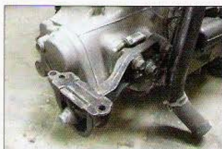
This front transmission bracket stabilizes the transmission during engine movement. Although some choose not to install it, it's highly recommended.
