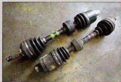
The two stripes shown in the middle of each axle designates the type of vehicle that they came from.
