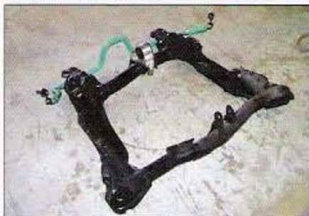
This subframe is from the RSX and is going to be installed on the Civic chassis. Attach the sway bar and rear mount before bolting it into place. (Photo Courtesy of Hasport Performance)
