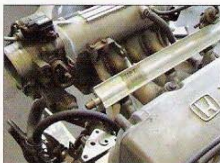
SOHC VTEC engines are easy to find, yet they aren't available out of that many different vehicles. This 125-horsepower example came from a '93 Civic Si.
