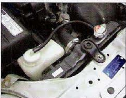
This Del Sol DOHC VTEC twin-core radiator is a must-have when installing the H-series engine. The original Civic unit is just too small and isn't up to the task.
