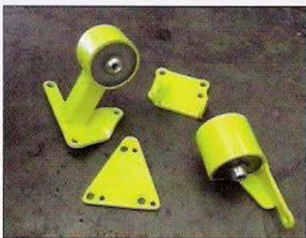
Unless you're up for quite a bit of welding, these specially designed engine mounts from Place Racing will be mandatory for the H series transplant.
