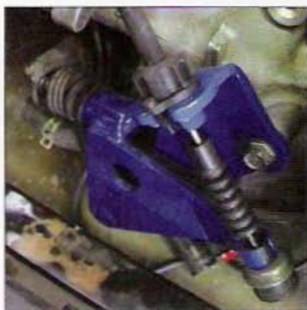
This cable-to-hydraulic actuator kit is a must-have for all H-series swaps into the '88-'91 Civic chassis. Notice how easily it bolts into place, allowing you to reuse the OEM clutch cable.
