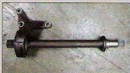
This is an early-style Integra intermediate shaft. This one can be used on any B-series swap provided you use the correct axles.
