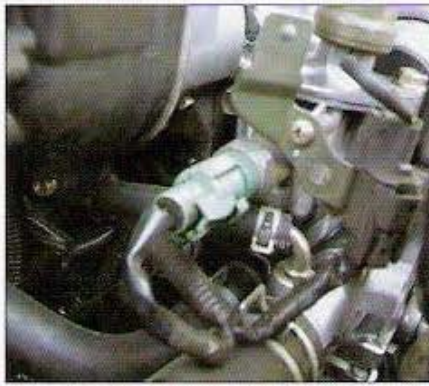
You must add wiring to the harness for the VTEC pressure switch shown here. The VTEC solenoid wiring is to its right.
