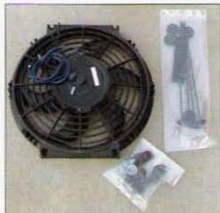
A smaller fan such as this will be mandatory because of clearance issues. You'll find that you can mount these on either side of the radiator since they can either pull or push.
