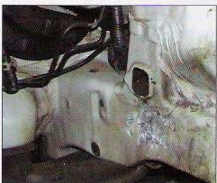
Right in the center of the photo, you'll notice where the frame was pounded for alternator clearance. This is another spot where it won't hurt to do too much.
