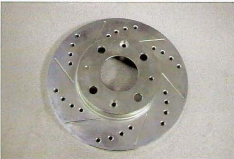
Cross-drilled and slotted rotors are an upgrade that you should look into when doing any engine swap. With all the extra power from the B series, it would be nice to know that you can stop it.
