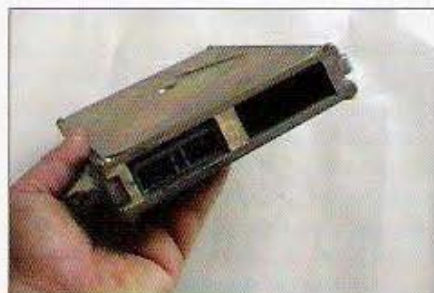
Most engines sold at a salvage yard will come with the proper ECU. If not, be sure to select the proper OBD 0 computer, as it will be necessary for the ZC engine to run properly.
