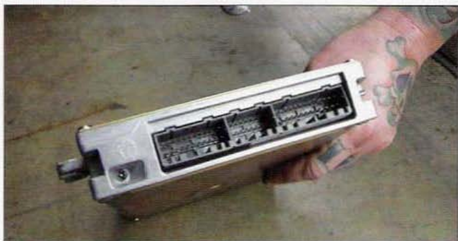
Ideally, this OBD I computer will provide you with the best results regarding performance. The OBD I units make the most sense since they can be reprogrammed easily.
