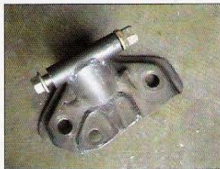
Up until just a few years ago, if you wanted an engine swap, you had to custom fabricate your own mounts, like this one. Luckily, several manufacturers produce engine-mount kits for almost any Honda engine swap.
