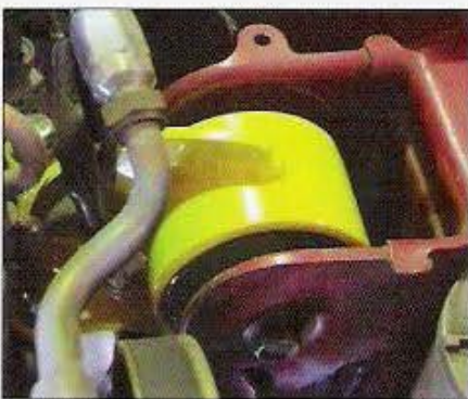
This Place Racing driver-side engine mount allows this whole procedure to be a bolt-in affair. Just think: this job used to require welding.
