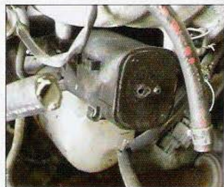
You must use this vacuum box when installing the IAB system for a Prelude engine. Be sure to find one that doesn't have snapped-off vacuum ports like this one (they usually do).
