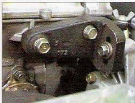
Matching the proper upper power steering bracket to your pump is mandatory. If you are looking for one in a junkyard, note the P72 stamped on the front of this one.
