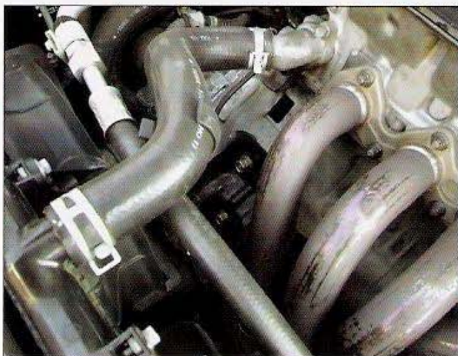
You can install a Prelude upper radiator hose to work with the original Accord radiator.
