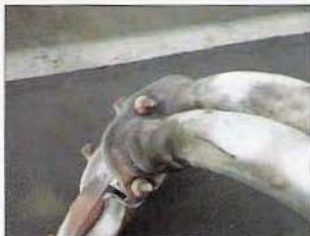
When selecting a B-series exhaust manifold, remember that almost all are compatible with any B engine. Be careful not to mix and match top halves and down pipes, as the later models are not compatible with the earlier. Try to find a complete unit.
