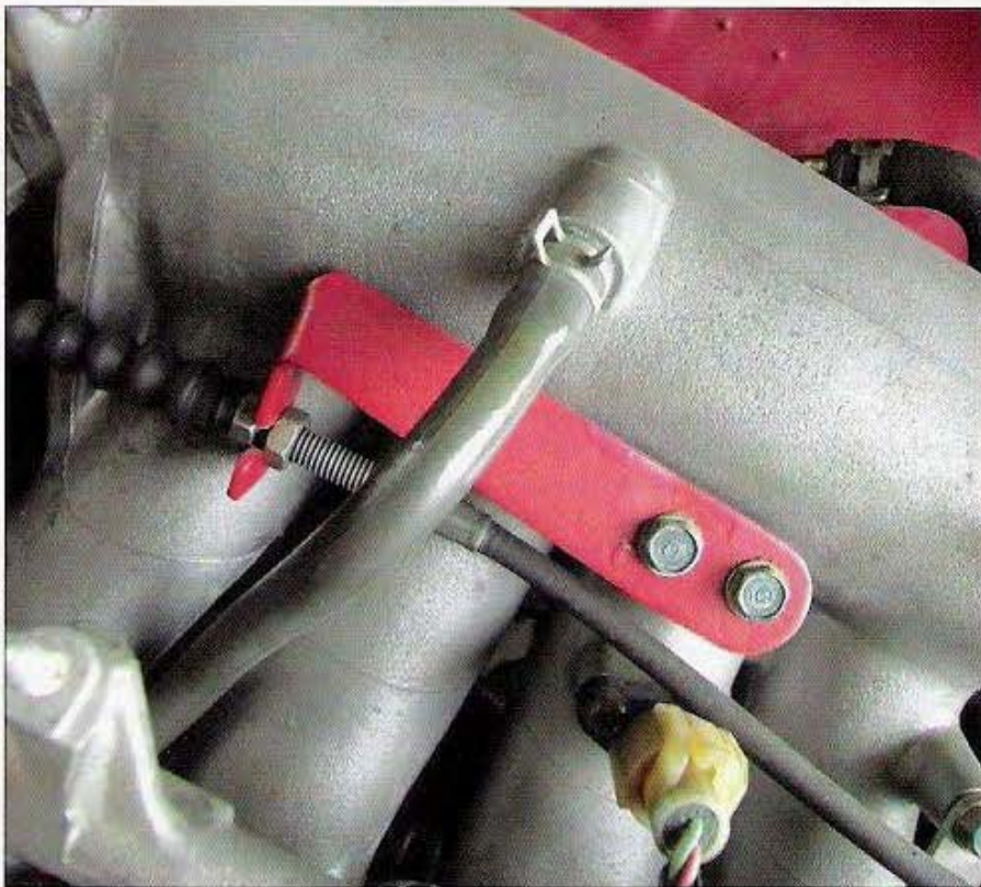
This special bracket from Place Racing allows you to reuse the original throttle cable on the Si models, which saves you from a bit of work underneath the dash.
