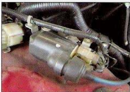
This external distributor coil will come in handy if you're using a USD M H22A1 engine with this type of setup. If so, simply plug the old coil wire into the new distributor.
