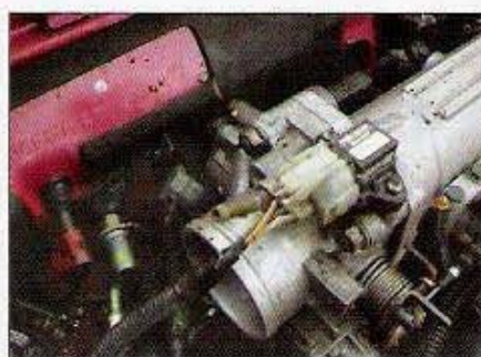
The new engine has its MAP sensor on top of the throttle body, so lengthen the appropriate wires from the vehicle harness to reach.
