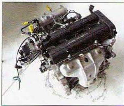
B20B engines are popular alternatives for enthusiasts who seek the maximum in engine displacement. Later you can install a VTEC cylinder head and have the makings for quite a bit of power.
