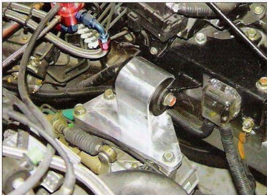
This Hasport Performance billet driver-side mount is about as strong as you can get. With the two side mounts in place, the engine will sit fine. (Photo Courtesy of Hasport Performance)
