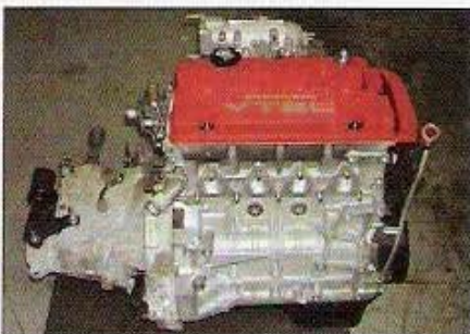
This H22A1 came from a '93-'96 Prelude Si VTEC. It's one of the largest engines that will fit into these chassis; it also has the most horsepower.
