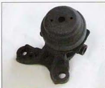
Install this Prelude driver-side mount on the left-side pocket mount in the '94-'97 Accord. Before you can do this, you'll need to cut down the bushing protruding out the right side.
