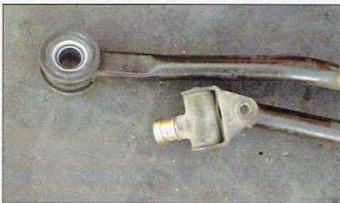
Custom shift linkage setups from Place Racing or Hasport Performance have OEM-looking ends that attach to the transmission.
