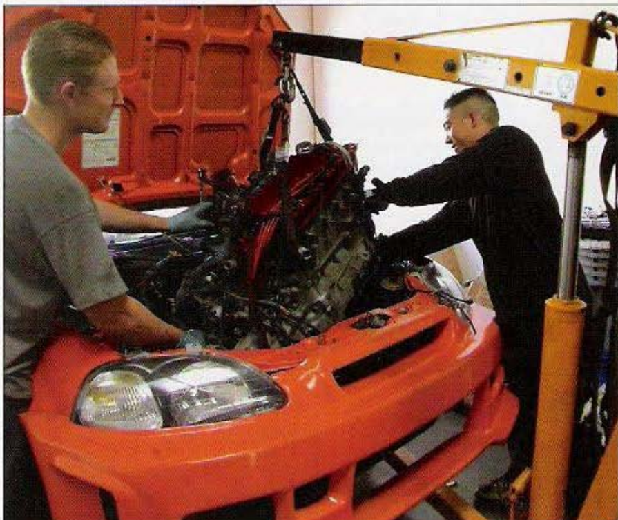
The guys at Import Life remove the old D series out of this '96 Civic, making way for a more powerful B16A.
