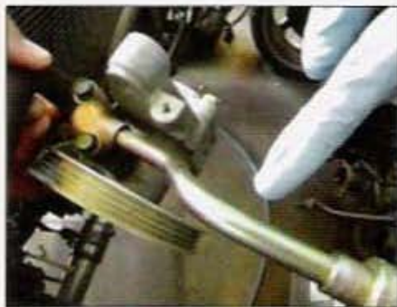
This is right where you want to cut the power steering line if you plan on keeping it. Once it's cut, the piece on the left can be discarded for a similar piece from a Prelude.
