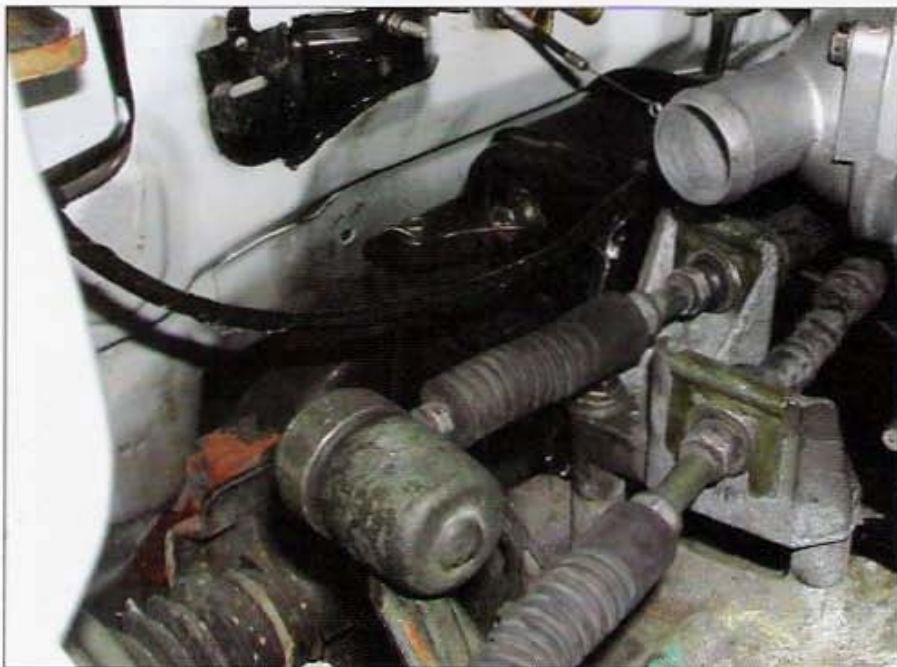
When reinstalling the shifter cables on the transmission, be sure to use all the factory-supplied washers and cotter pins.
