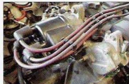
The cylinder position sensor runs off the exhaust camshaft on the ZC engine, as opposed to inside of the distributor on most others.
