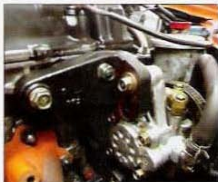
This power steering pump is a straight bolt-on process if you use the proper Integra components. Use an Integra belt here as well.
