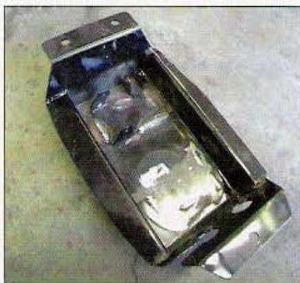
This adapter box from Place Racing allows you to eliminate the Prelude or Accord shifter plate. Bolting this to the underside of the car hides the cables away.
