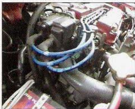
The distributor plugs shown here are just one example of several connectors that need to be swapped out for those of the B-series donor engine.
