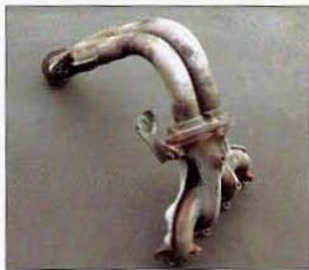
Although the original Civic exhaust manifold will bolt into place, this late-model unit from the D16Z6 VTEC engine will provide the utmost in OEM performance.
