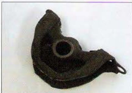
Do not remove these special rubber engine vibration mounts from the vehicle. The Integra versions are not compatible with the Civic and vice versa.
