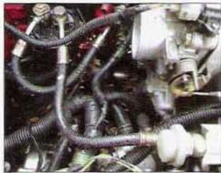
Swap the proper fuel injection feed line into place for the fuel system to work properly. The old line was incompatible with the damper pulsation nut shown here.
