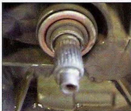
Depending on which year of Civic transmission you're using, these splines will differ slightly in their number and diameter. Make sure all your components match up when you're mixing and matching.
