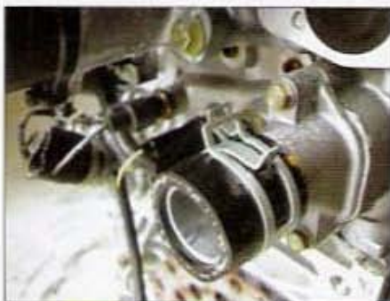
This water outlet on the B20B illustrates the larger diameter of the B-series radiator hoses compared to the Civic hoses. The Civic radiator has smaller inlets and outlets than this water neck.
