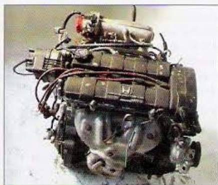
This is one of several JDM ZC engines that you may encounter at your local engine yard. Pay attention to the location of the driver-side engine mounts to be sure you're getting the proper one. Make sure it's on the front, not on the side.
