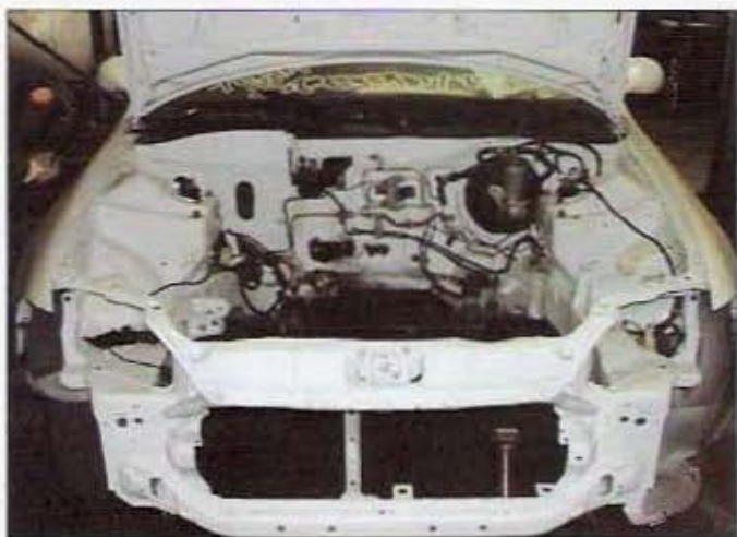
Stripped of its body panels, this Civic looks somewhat similar to the third-generation Integra. This is one reason why the Integra engine swaps into these '92-'95 Civics are so basic.
