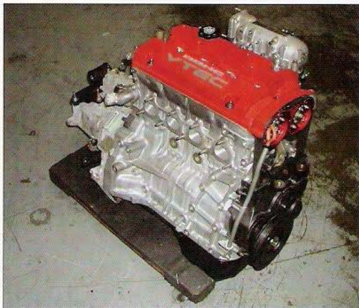
This JDM H22A engine is a perfect donor engine for these vehicles, as it is a direct bolt-in fit.
