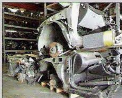
Many engines arrive from Japan in the form of a front half of a car, otherwise known as a clip. These are cut in two and shipped throughout the United States.
