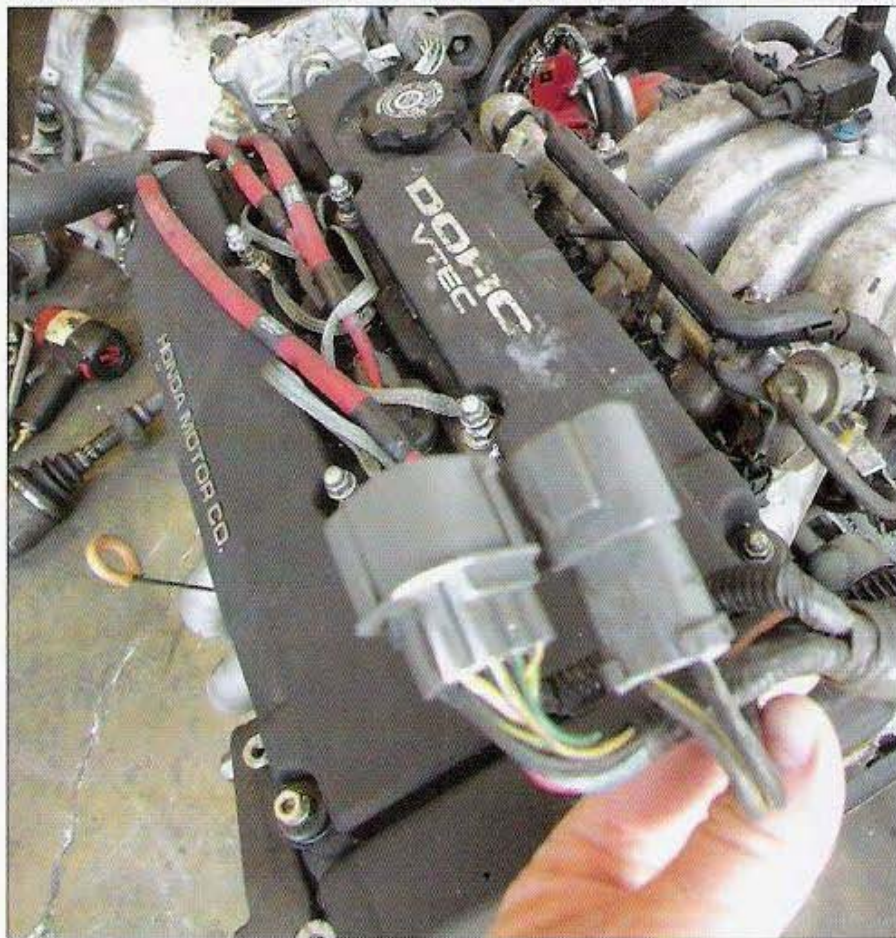
When trying to finagle a JDM-style engine harness to a USDM vehicle, you'll find it'll cost you hours of unnecessary labor. Since the JDM harness is designed for right-hand drive, the harness will be almost a mirror image of its USDM counterpart.
