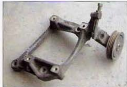
If you're using the HCP Engineering bracket when reinstalling you're A/C, keep the original pulley and bolt because they will be reused.
