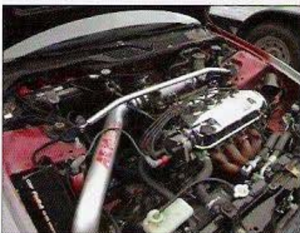
The D16Z6 is one of available several factory engines for this Civic. Out of all of the available SOHC Honda engines, this is one of the more powerful and most upgradeable.
