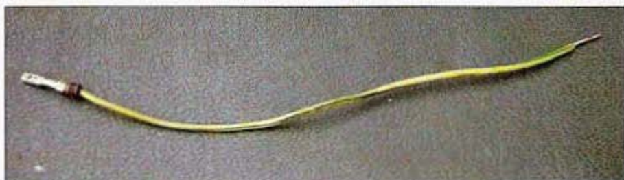
When you move plugs around and add wiring to the harness, using pins like these in the plugs will give you a more factory look as opposed to cutting and soldering.
