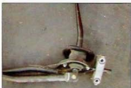
This shift linkage mechanism from the Integra will provide a factory bolt-on fit without any modifications. The Civic unit is worthless here.
