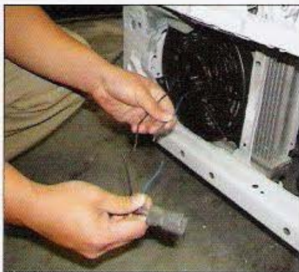
Notice how the smaller radiator fan sits perfectly in the space between the bumper and the radiator. Simply connect these two wires to the appropriate locations the same way the old fan plug was connected.
