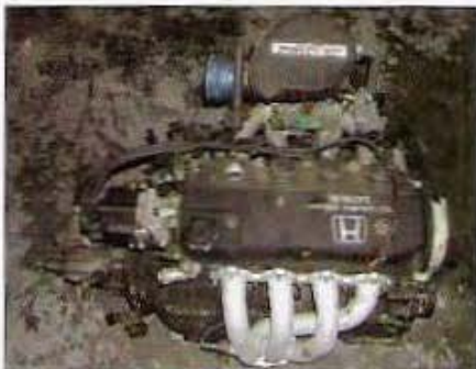
These dual-injected D-series engines are worthless as far as horsepower is concerned. The money spent on this header would be better used on an engine swap.
