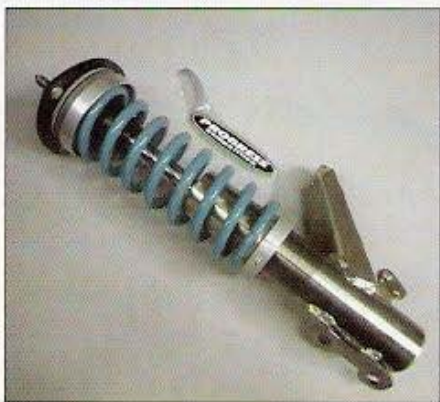
Coil-overs from the folks at Progress Suspension will allow you to fine-tune the front and the rear of the vehicle to suit your needs. This is helpful when you install the much heavier Prelude engine.
