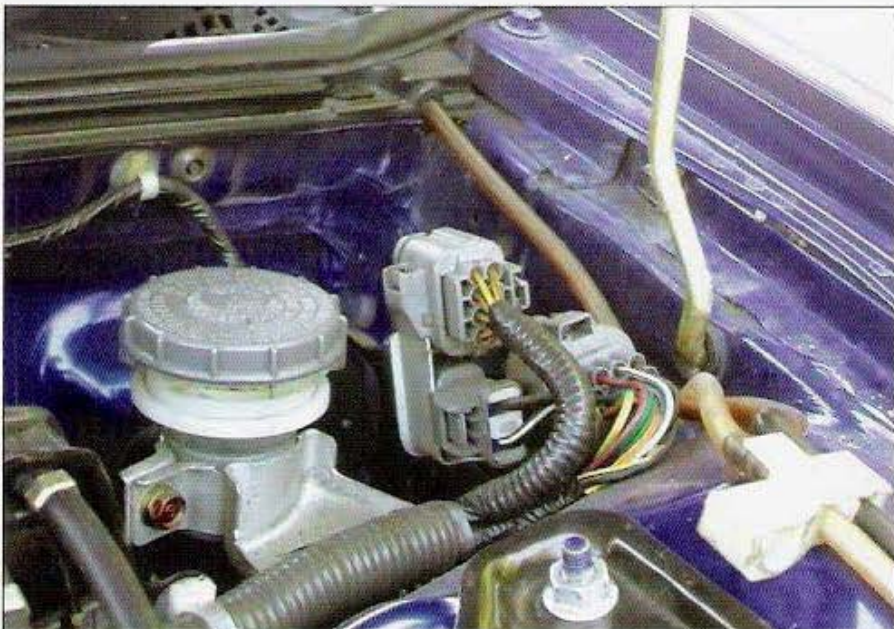
Using the original engine wiring harness of your vehicle when doing an engine swap will save you quite a bit of work. Once you get properly hooked on to the new engine, you'll find that it will plug right back into your vehicle.
