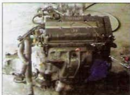
This JDM B16A engine is as complete as they come. Notice how it is equipped with a complete exhaust manifold, both radiator hoses, and of course, the transmission. The distributor has been removed so it doesn't get damaged.
