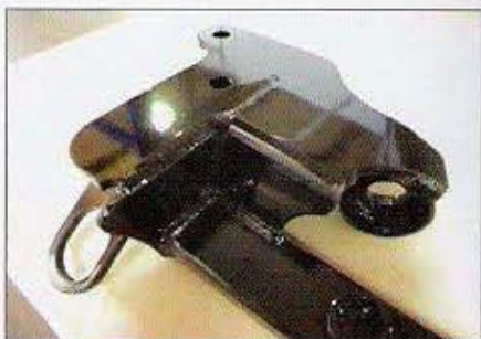
This Place Racing crossmember is designed for use with the H-series engine. You'll find that it easily bolts onto the factory locations.
