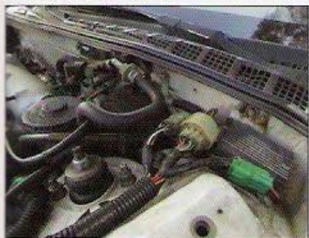
If your engine doesn't already have one, you'll need to mount an injector resistor box in the factory location up in the driver-side corner of the engine bay. Some dual-point engines don't come with them.
