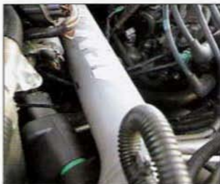
This external coil on the '94-'97 Accord is retained so that it may be reused with the external-coil distributor of the USD M Prelude H22A engine.
