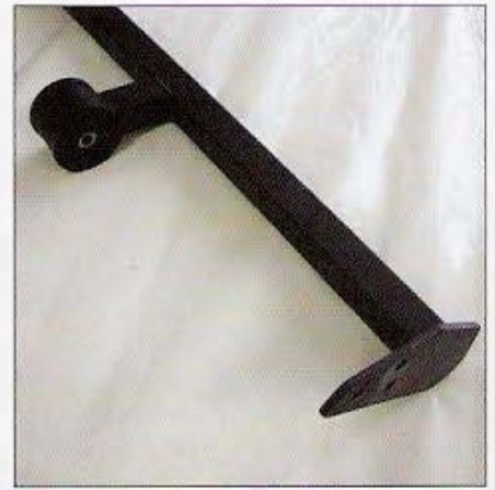
Many engine mount kits are equipped with a custom front crossmember such as this unit from HCP Engineering. These are a good idea since they're designed to help stabilize the more powerful engine.
