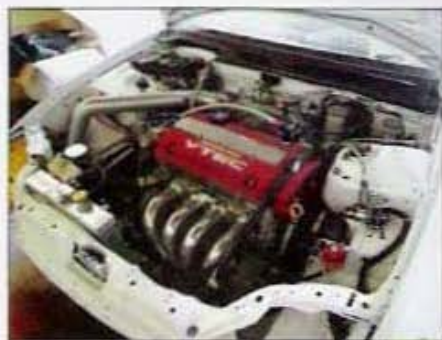
Once you get it finished, you'll find that the Prelude engine sits quite snugly under the hood of this Civic. There will even be plenty of room left over for a custom header such as the one shown here.
