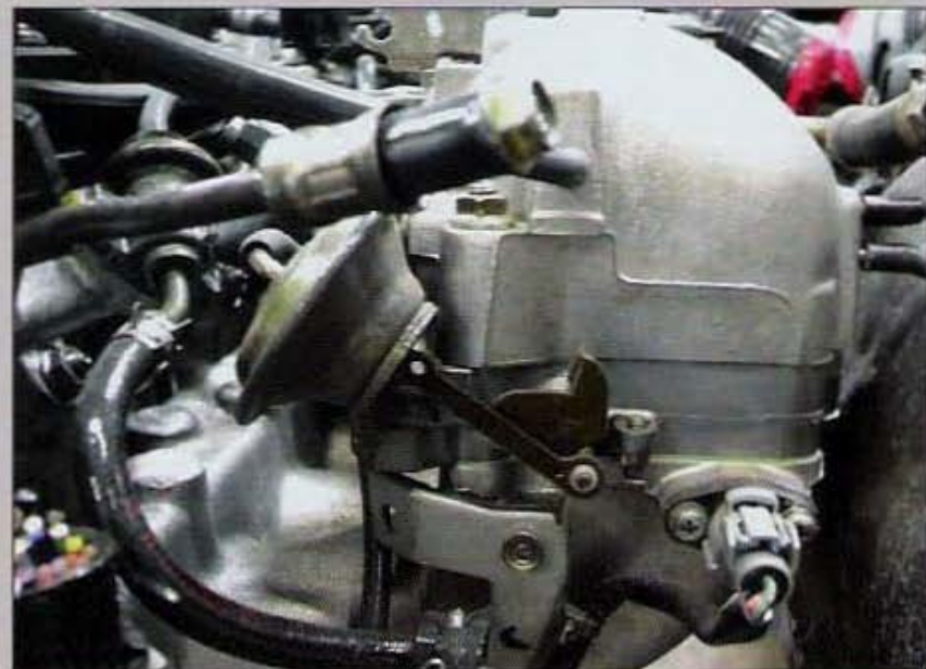
Notice the stacked manifold design. These secondary-type intake manifolds are actually three pieces bolted together.
