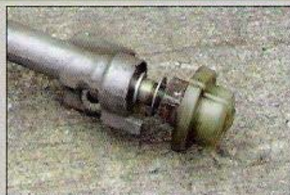
This damper pulsation nut assembly is more common to newer vehicles, although it can be found on select Si models all the way back to 1986.
