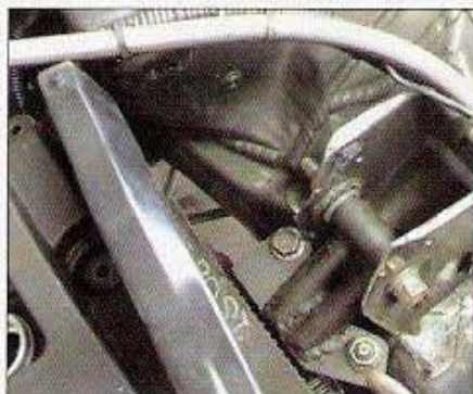
Many folks choose to manufacture their own custom mounts in lieu of the Place Racing kit. Either way, welding is going to be required.
