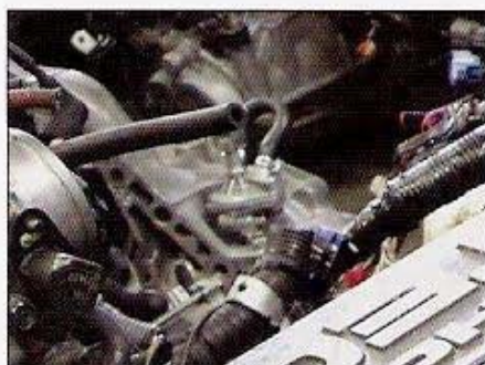
The H22A1 Prelude VTEC engine is the most common H swap for any chassis. In this photo, you can get a good view of the secondary-type intake system of the Prelude intake manifold.
