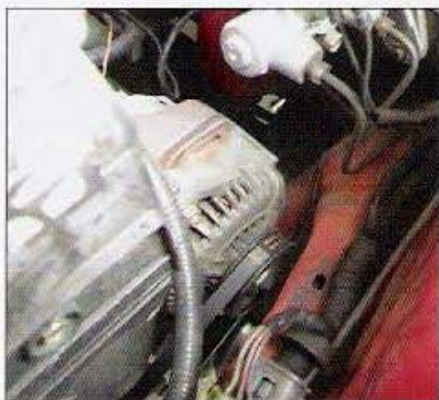
Alternator clearance is at a bare minimum. Installing a slightly longer belt will require you to adjust the alternator back closer to the frame, which is a bad idea.
