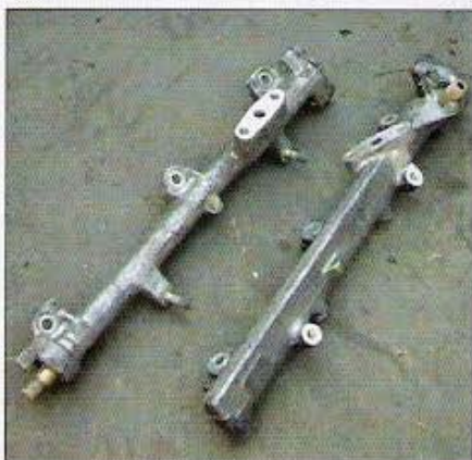
Here's a comparison of the two different types of Prelude fuel rails. The unit with the fuel feed port on the passenger side (on the left) works best on the Integra.
