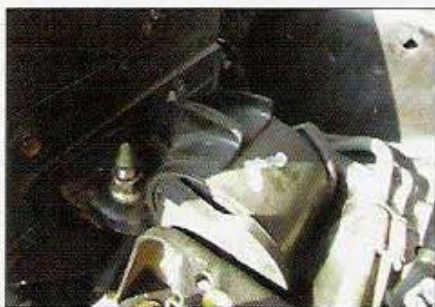
Certain Civics and Del Sol's use this different left-side mount. You need to install a different post bracket on the block if you're going to use this mount.
