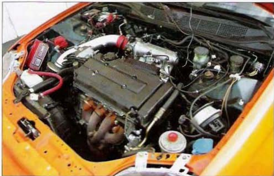
Similar to what you would find underneath the hood of the '99-'00 Civic Si, the B16A provides you with the most factory fit that you could hope for from an engine transplant.
