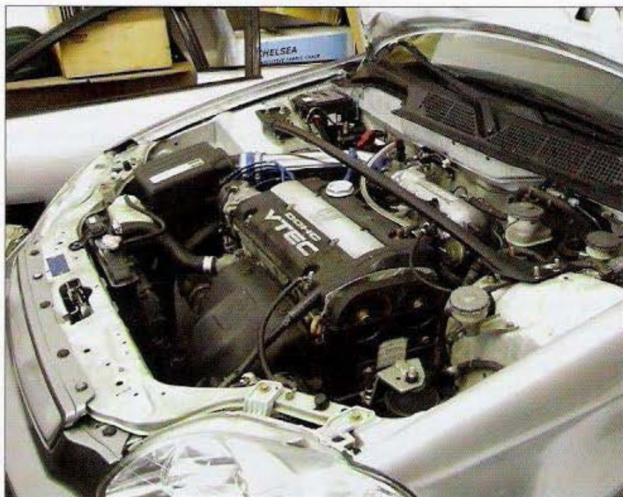
Although it's time consuming to say the least, few swaps provide the enjoyment that an H series does. Once installed properly, you'll find that it fits snugly right under the Civic hood.
