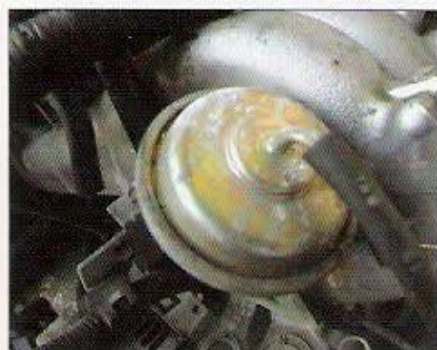
The intake air bypass valve found on the later-model GSR engines is an optional hook up. Although it isn't difficult to wire into place, the IAB won't pose a problem if you leave it unconnected.
