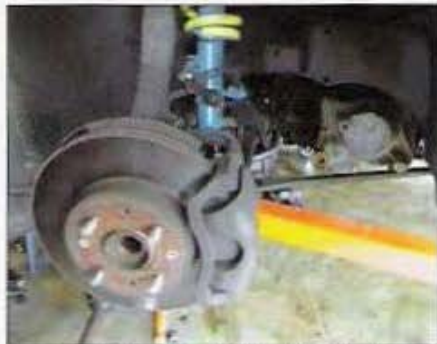
These '88-'91 Civic EX knuckles, hubs, rotors, and calipers were installed for extra braking. This is another bolt-on procedure for the Civic.
