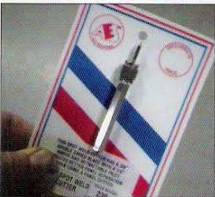
Remove the factory spot welds in a clean and quick manner using this special drill bit from Place Racing.
