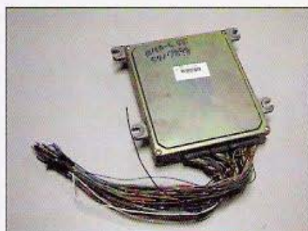
This JDM ECU is smaller than the USDM version, which makes it an easy find. This particular computer is already equipped with the plugs necessary for the OBD conversion.
