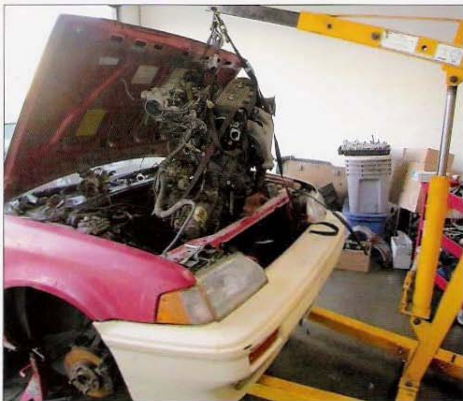
The useless SOHC engine is being hoisted out of this first-generation CRX to be replaced with a larger and more powerful B series.
