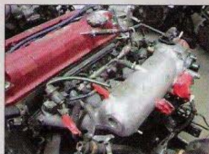
Notice the tape that covers up the fuel return line, the vacuum ports, and the throttle body. You might want to think twice about purchasing an engine with openings that expose the internals to the elements.
