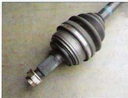
Specially designed axles will be necessary due to the differences in hub diameters. Notice how this axle has the smaller, Integra type of splines.
