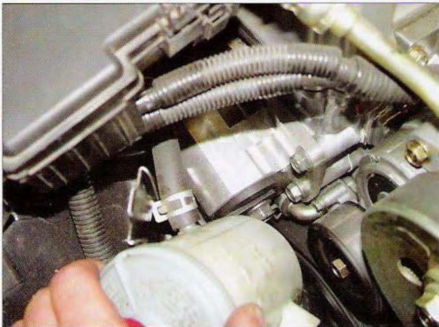
You can solve your power-steering reservoir problem by using one from an older Civic. It can be slid into place and will work fine. (Photo Courtesy of Hasport Performance)
