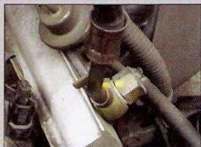
This standard cap nut assembly is found on many base-model Hondas and most older vehicles.
