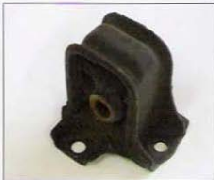
Reuse this Accord front mount along with its corresponding bracket. The stiffer Prelude units are not compatible with the Accord crossmember.
