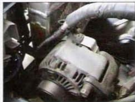
Notice the tight fit between the radiator and the alternator. If you push it a bit farther backward, there'll be just enough room between the two.
