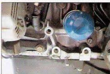
Since all ZC engines have provisions for an intermediate shaft, you'll need to make sure you pick one up from the junkyard when you bring the engine home. The 3 empty bolt holes that you can see around the bottom left of the blue oil filter are for the halfshaft.
