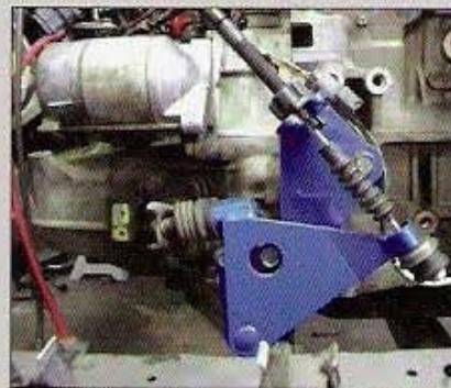
Notice how the Place Racing conversion bracket bolts right to the front of the engine and reuses the original clutch cable.
