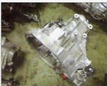
You can identify cable-style transmissions by the bolt pattern for the top mount. The cable-operated arm in the upper portion of the photo also gives it away.
