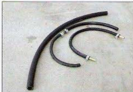
When making a custom fuel line, be sure to use fuel injection hose and hose clamps to ensure a leak-free setup.
