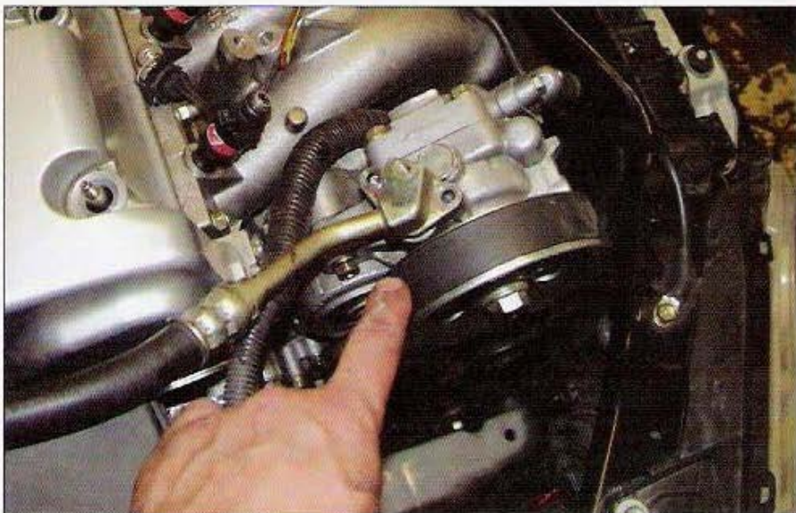
The power-steering line from the RSX is used to attach to the RSX power-steering pump. It bolts into place with the right components. (Photo Courtesy of Hasport Performance)
