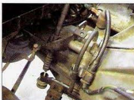
The original cable-style Civic transmission is perfectly compatible with the newer engine. Reinstalling it is a simple bolt-in procedure.
