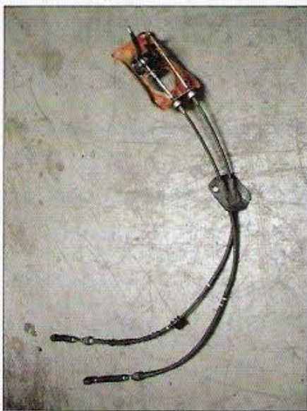
These shifter cables from a late-model Prelude are necessary since the original ones aren't long enough.
