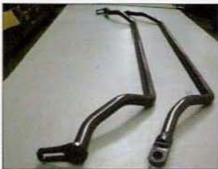
This larger diameter anti-sway bar on the left from Progress Suspension is necessary for all Prelude engine transplants. It's a good investment because it helps to alleviate understeer.
