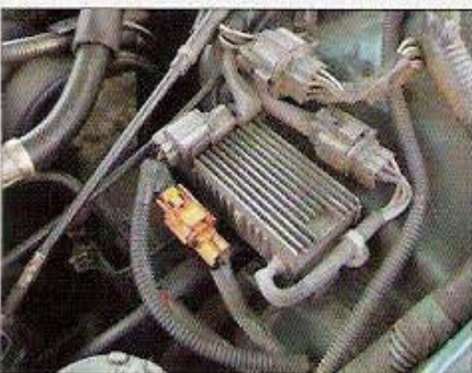
When dealing with OBD I Integras, a resistor box such as this one will need to be added. Either bolt it in place or zip tie it somewhere safe once it's wired up.
