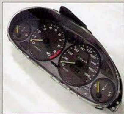
This JDM gauge cluster is a perfect post engine swap addition. Notice that the tach reads up to 10,000 rpm and that the speedometer reads in km/hr.
