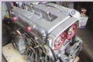
The front of the engine is actually the side that houses the camshaft gears, timing belt, and crankshaft pulley, all of which you can see here.
